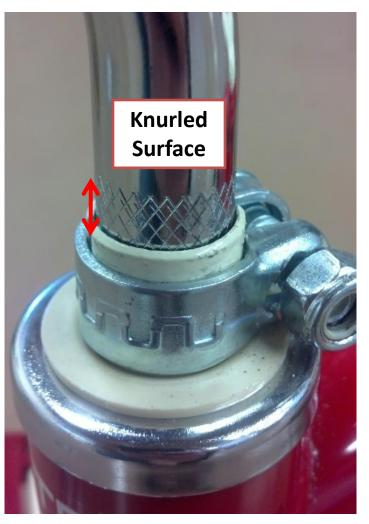
Slide the clamp over the fork. Insert the handle bar into the fork while leaving a ¼" of the knurled surface exposed.
