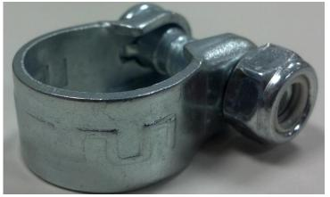
Insert the bolt into the clamp. Line up the notch on the bolt with the keyway on the clamp.
