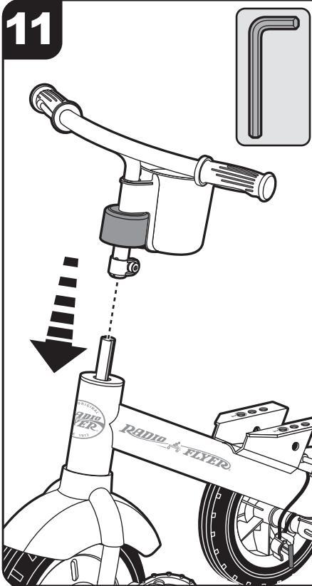
Make sure the handlebar is fully inserted into the stem, then tighten the fork clamp until the handlebar is secure.
