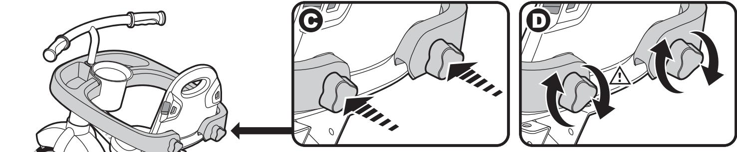
**⚠ Warning:** Do not lift tricycle by the safety arms. Make sure rear knobs are fully tightened before use.
