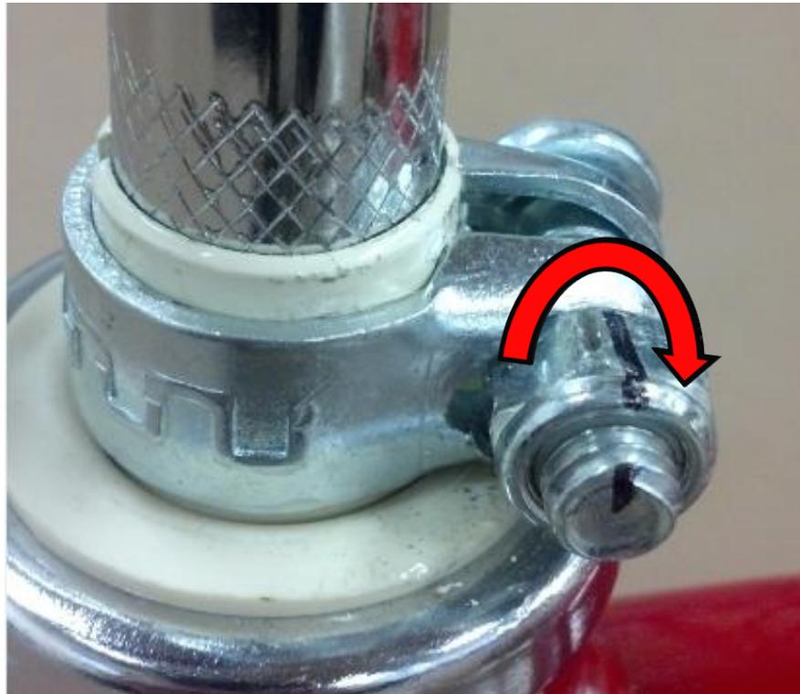
Turn the nut 3 full rotations to ensure proper assembly.
