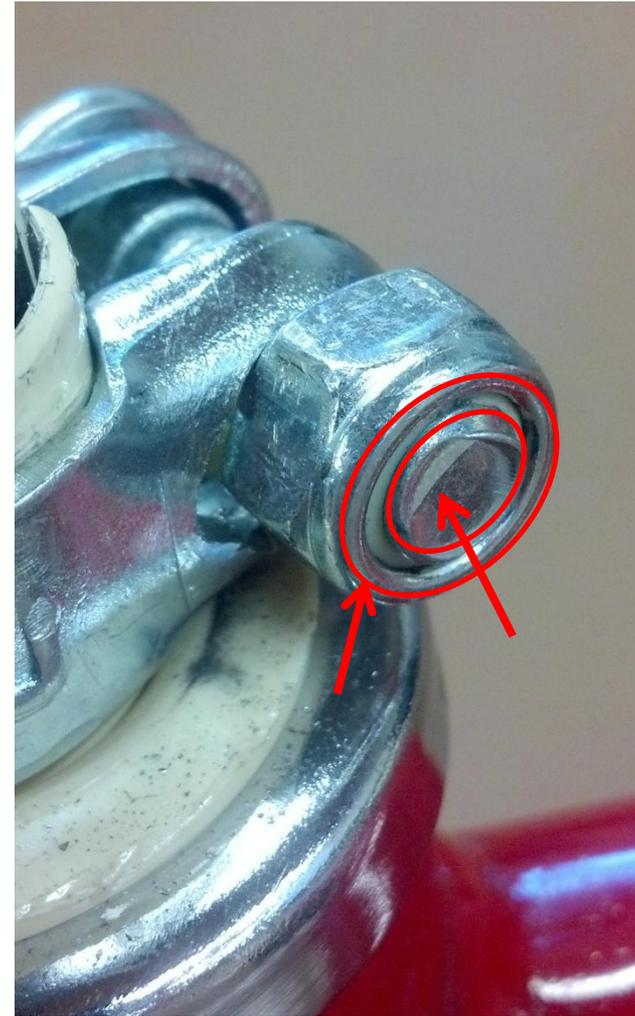
**Tighten the bolt until the outer face of the nut and end of the bolt are aligned.**
