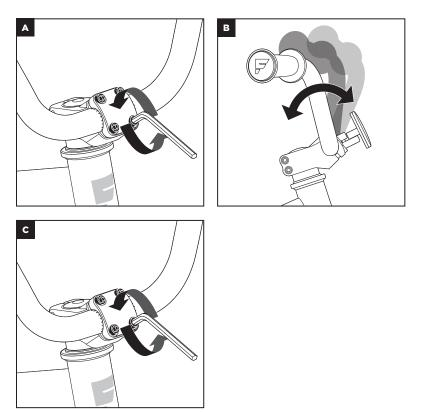
A WARNING! The stem on your Flyer<sup>™</sup> kids' bike comes factory assembled to the front fork, and does not need to be removed to adjust the handlebars. If the stem is loosened or removed from the fork, care must be taken during re-assembly to avoid damaging the stem-to-fork connection. Overtightening the stem clamp bolts can damage the stem-to-fork assembly, which can lead to risk of injury. To avoid overtightening, use a torque wrench to tighten the stem clamp bolts to 18 to 20 Nm.
