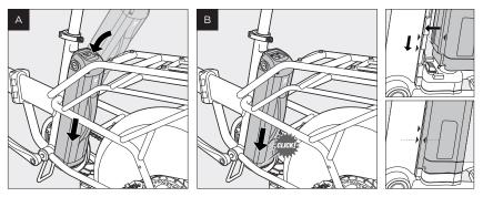
A WARNING! Always lock the battery in place before riding. Failure to lock the battery could cause damage to the bike.
