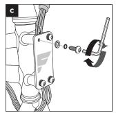
Note: Following installation of the front logo plate, check that the cables and wires can move freely by turning the handlebars fully to either side. If any resistance occurs, the wires and cables should be repositioned by sliding them up or down along the headtube.
