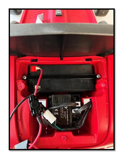
Connect the new battery to the PCBA and the harness.
