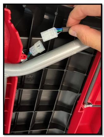
Disconnect the direction switch from the pedal.
