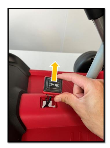
Insert the new direction switch into the car. Note, the blue wire should at the front of the switch (toward the front of the car) when installed. Incorrect orientation will result in reversed function.
