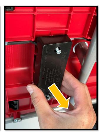
Remove the 3 strain reliefs fastening the wires for the direction switch to the bottom of the car.
