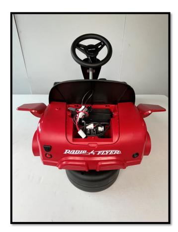
Once the axle has been removed, the motor and cover should drop out.
