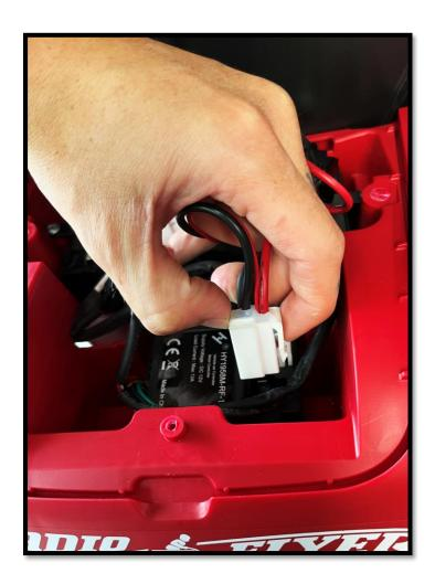
Disconnect the motor you are replacing from the PCBA.
