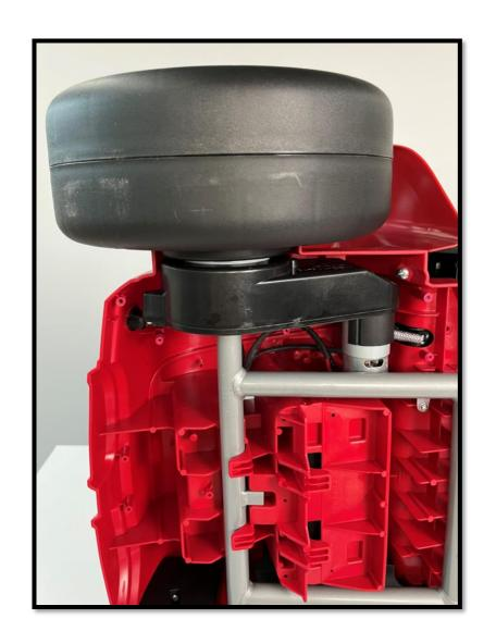
Flip the car upright. Use a flathead screwdriver to pop the cover of both rear wheels.
