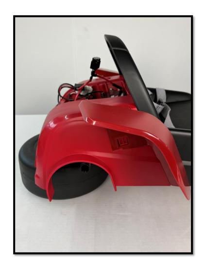
Insert the new motor into the motor cover.
