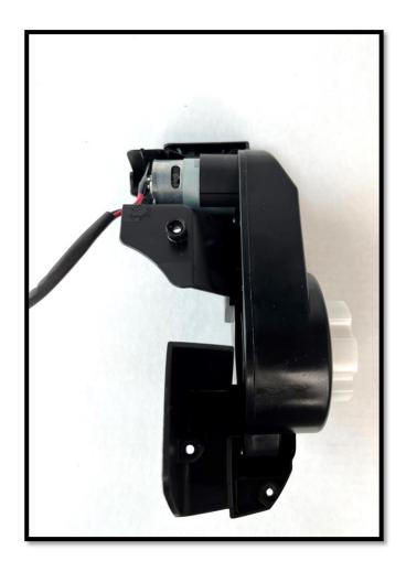
Route the wire from the new motor through the opening into the rear bin.
