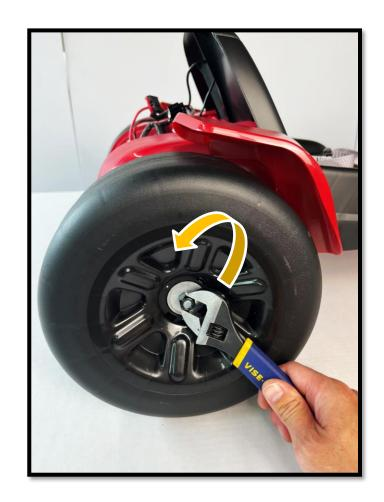
Remove the wheel on the same side which the motor is being replaced.
