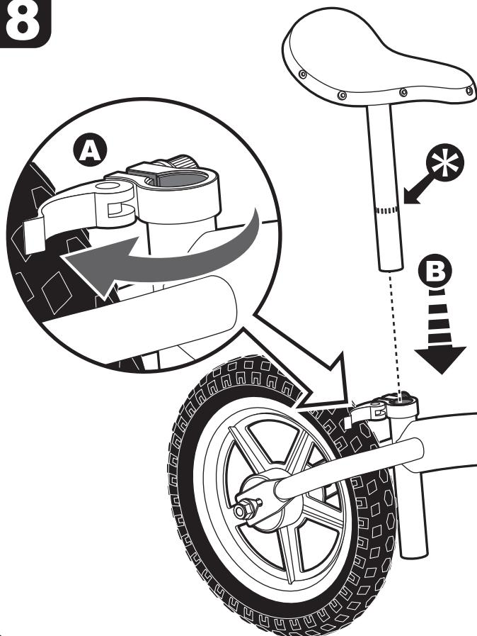
**Insert seat post into frame to, or past the minimum insertion mark shown on the seat post and then tighten the frame clamp until the seat post is secure.**
