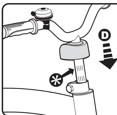
!\* Insert handle stem into fork to safety mark and then tighten handle clamp until handle is secure.
