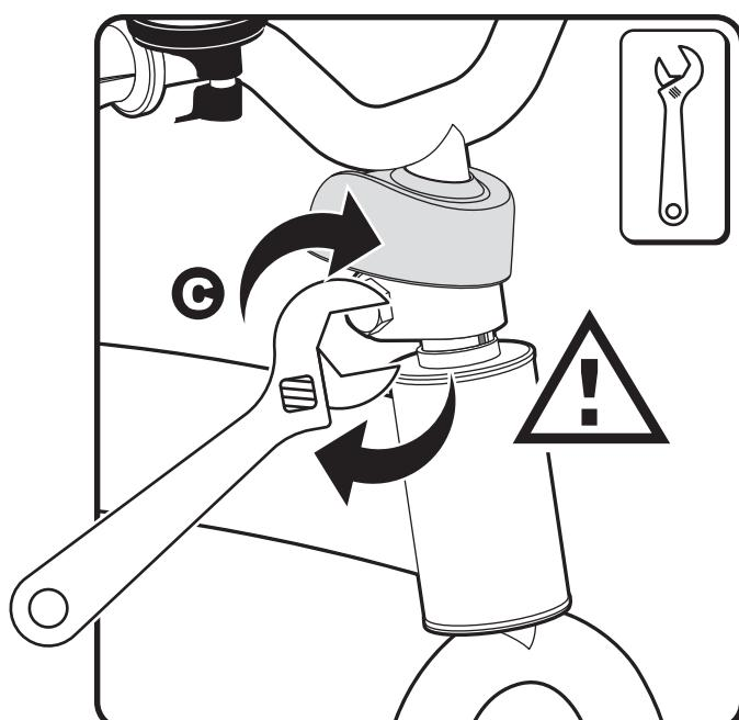
!**CAUTION:** Be careful not to over tighten the handle clamp, causing the bolt or nut threads to strip. This could lead to stem-to-fork failure and result in a risk of injury to the bicycle rider.
