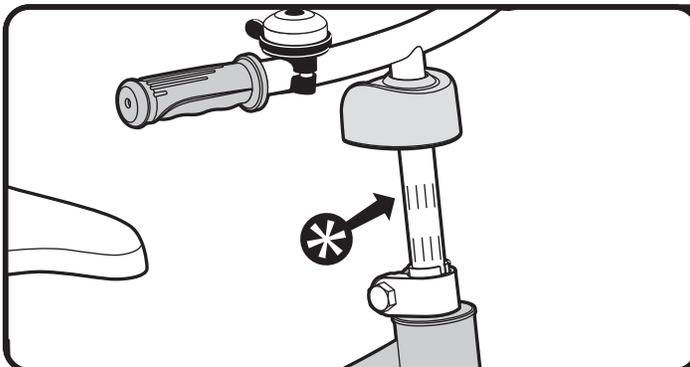
✳ Insert handle stem into fork to safety mark and then tighten handle clamp until handle is secure.
