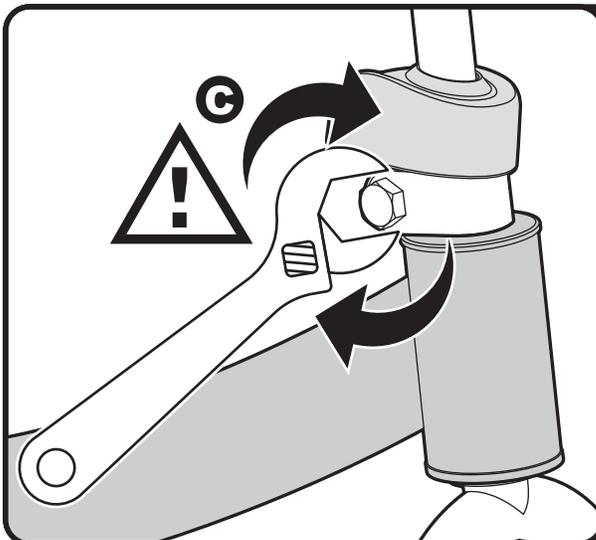
⚠ CAUTION: Be careful not to over tighten the handle clamp, causing the bolt or nut threads to strip. This could lead to stem-to-fork failure and result in a risk of injury to the bicycle rider.
