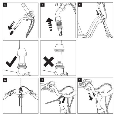
Note: Complete assembly of the bike per the steps below. The stem and handlebar angle can be adjusted as needed based on rider preference. Always re-tighten bolts to the specified torque values prior to riding.
